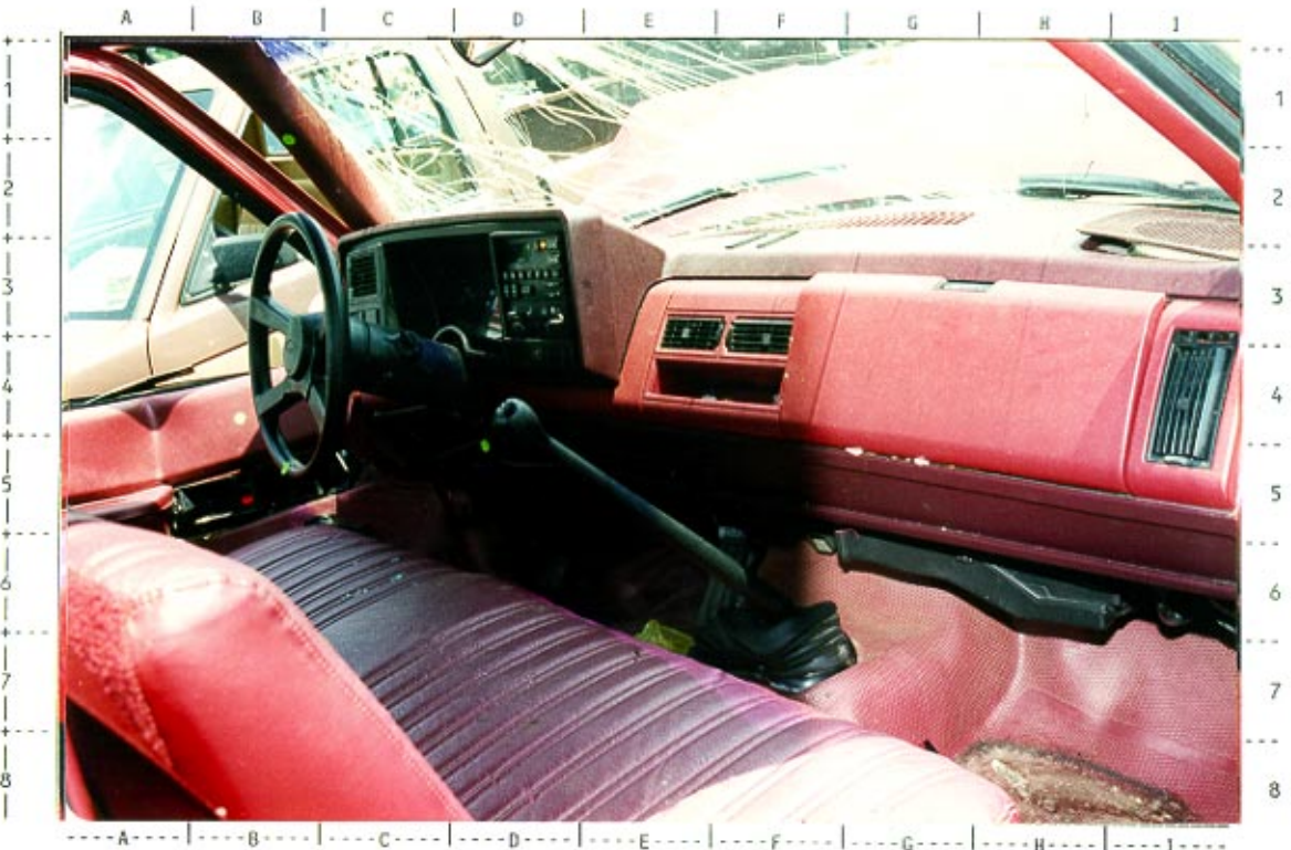
# 90 -- Steering wheel & dash of 1988 Chevrolet pickup viewed from right exterior; NOTE: evidence of driver contacts (dots) on left dash
